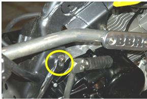
8. Remove center engine bolt.
