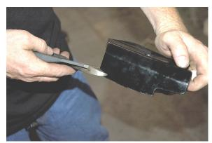
**12.** Trim counter shaft sprocket cover for shock tower clearance.
