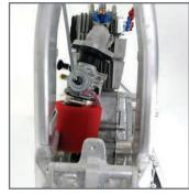
Also uses the supplied manifold adapter. Set adapter offset to the left with the throttle cable running between the frame spar and gast tank.
