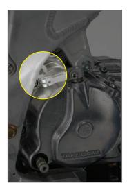
If you are using the Takegawa Manual Clutch, you will need to use the supplied clutch cable stop located on the frame.
