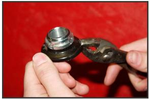
**11.** The upper dust seal will require modification to fit the large headtube of the BBR frame.
