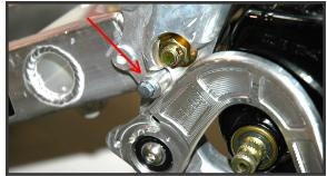
**17.** Use brake adjuster cam to set the height of the brake pedal when using the drum brake.
