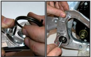
8. Install the brake pedal by inserting the brake pedal spring into the brake pedal first, then install the assembly onto the frame.
