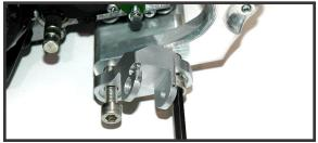
**9.** Install the footpeg mounts and then install the footpegs onto the mounts. Note that these mounts only fit KLX110 specific footpegs.
