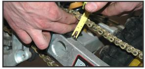
**Chain Adjustment:** Adjust the chain so that it has about 1.5 inches of play at the end of the chain buffer block.
