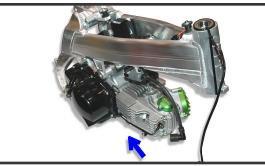
**5.** Install motor by sliding up into frame centering bottom motor mount plate between the bottom frame spars.
