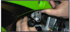
If you are using the stock carb, install the choke with the supplied mount as shown above. We recommend changing to a #98 main jet (BBR #421-KEH-3098)
