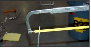
**15.** Carefully cut brake rod (we recommend using a hack saw) leaving 3/4" of threads then install the brake rod adapter as shown.
