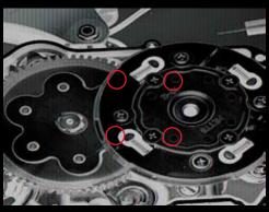
**15.** Straighten the tab of the clutch lock nut lock washer. Remove the clutch lock nut with the appropriate special clutch tool. It is available from Honda as part #07716-0020100.
