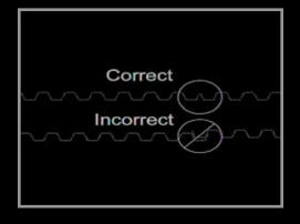
20. Install a piston clip into the piston. Use your fingers to compress the rings while sliding the piston into the cylinder. Turn the piston so that the "IN" is facing the carb/intake side of the cylinder. Let the piston protrude enough to insert the piston pin.
