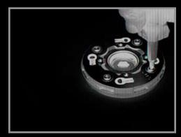
**5.** Remove the (4) 10mm nuts from the top of the cylinder head cover and remove the cover.
