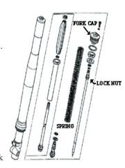
Check to make sure your oil level is 95mm. Please see your owners manual for instructions on doing this. Tighten the fork cap onto the lock nut to 14 lbf-ft. Thread the fork cap into the fork tube and torque to 25lbf-ft.Reset the rebound adjuster screw position and reinstall the forks. Torque the fork tube pinch bolts to 16lbf-ft.
