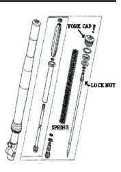
Check to make sure your oil level is 95mm. Please see your owners manual for instructions on doing this. Tighten the fork cap onto the lock nut to 14 lbf-ft. Thread the fork cap into the fork tube and torque to 25lbf-ft.Reset the rebound adjuster screw position and reinstall the forks. Torque the fork tube pinch bolts to 16lbf-ft.
