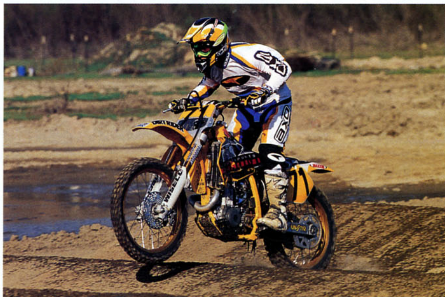
Stadium-style whoops would normally be the DR-Z's biggest nightmare, but Taylor proves that with an RM250 fork and shock, the bike is capable of tackling the roughest terrain.
