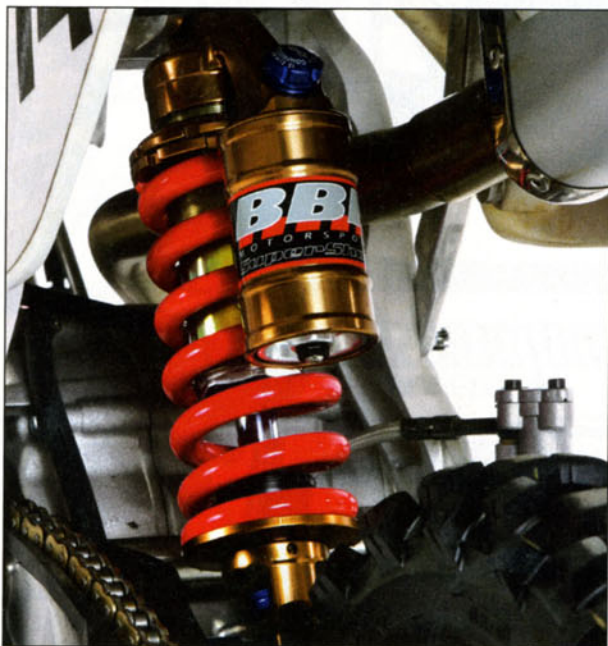
In order to complement various size pilots, the shock has two mounting positions for different ride heights.
