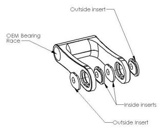
Align insert hole with swingarm linkage. This is easiest accomplished by raising or lowering the swingarm and the BBR linkage until they line up. When holes are aligned install outside insert and bolt through BBR linkage and swigrm linkage. Install other outside insert and nut.
