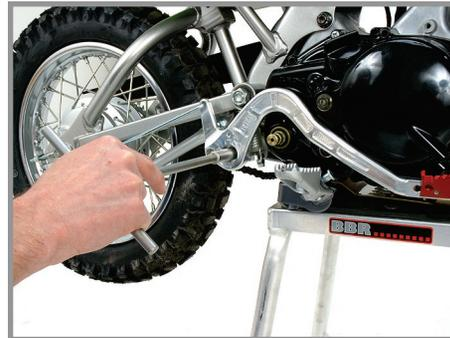
5. Install the brake pedal (tighten 10mm bolt to 79 in lbs). Be sure to hook the return spring on the frame.
