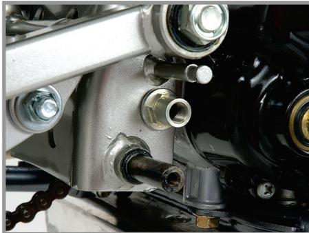
2. Replace the lower rear motormount bolt's nut with the special nut included in this kit (torque to 40 ft. lbs).
