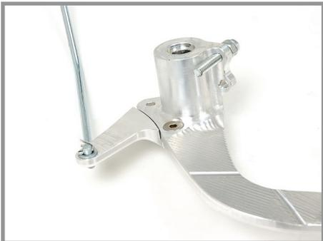
3. Install the brake rod into the BBR brake pedal and reinstall the cotter pin.
