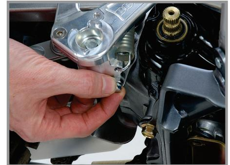
6. Adjust the brake pedal tip height as desired and lock the adjuster bolt in place.
