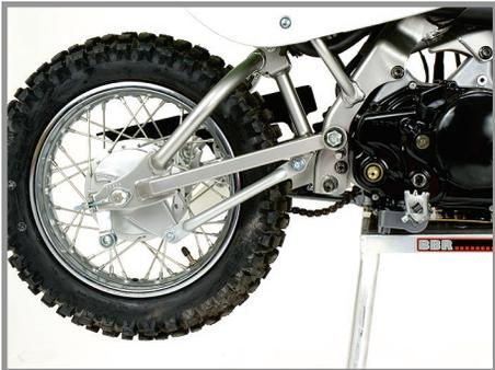
1. Place bike on stand and remove stock brake pedal (10mm bolt), brake pedal rod, and kickstarter.
