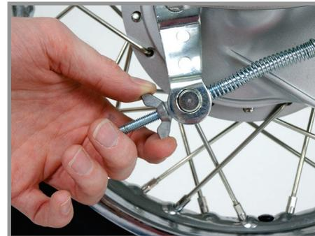
7. Reinstall the pull rod and adjust rear brake as desired. Standard adjustment is about 3/4 inch of pedal free play.
