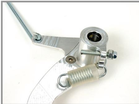
4. Hook brake pedal spring on the brake pedal. Install the stock o-rings in the BBR pedal.
