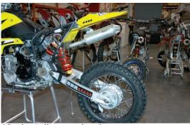
**13.** Install rear wheel using supplied M12 Fuji Locknut on OEM axle.
