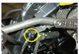
8. Remove center engine bolt.
