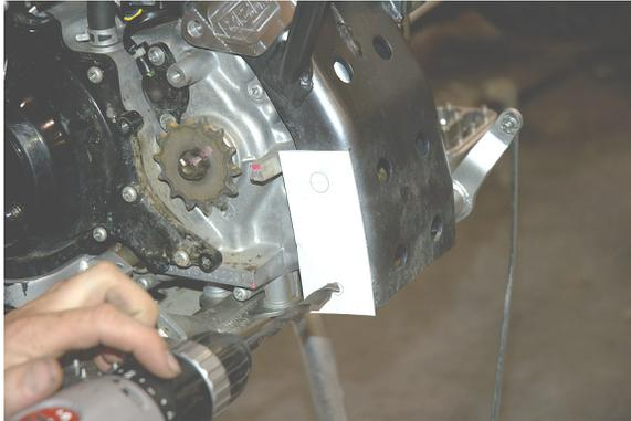
6. Drill frame for chain roller using the provided template to locate the hole (Non-L models only).
