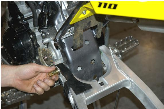
7. Install new swingarm (we recommend greasing the pivot bearings with a high quality water proof grease).
