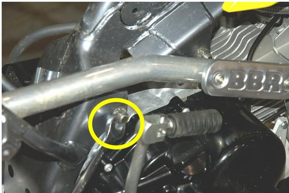
8. Remove center engine bolt.
