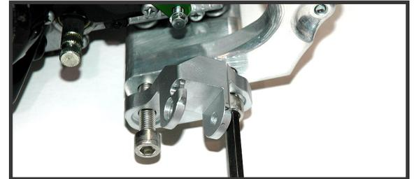
**9.** Install the footpeg mounts and then install the footpegs onto the mounts. Note that these mounts only fit KLX110 specific footpegs.
