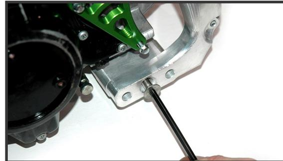
**7.** Install the 2 bottom motor plate bolts through the frame spars into the motor plate. Once all the bolts are installed, you can tighten all the motormount bolts. Note that these bolts should be loosened or removed when removing the swingarm. Swingarm bearings are pre-greased from BBR.
