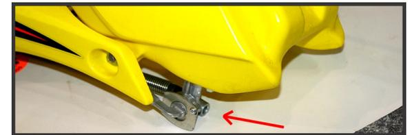
18. Install the gas tank using the fuel petcock and fasteners from the stock tank. Note when installing the tank shrouds, the lower wing mount hole will need to be pulled into place. This will put tension on the wing and hold it in place.
