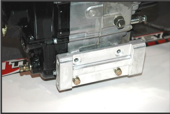
**3.** Attach the bottom motor mount plate to the engine (2 rear bolts). Note that the printing should face up and forward. Leave bolts loose.
