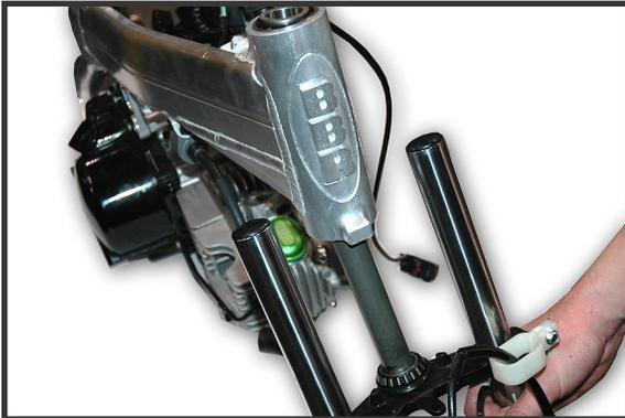
12. Install the triple clamps and fork legs (see last page for diagram).
