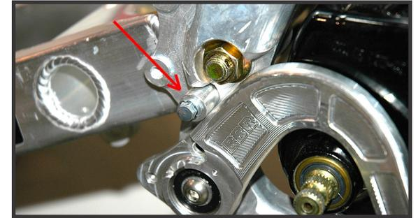
17. Use brake adjuster cam to set the height of the brake pedal when using the drum brake.
