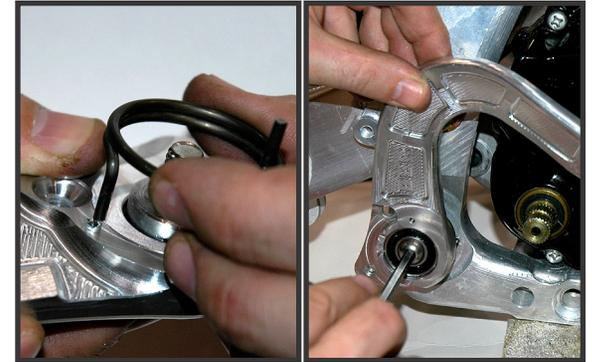
**8.** Install the brake pedal by inserting the brake pedal spring into the brake pedal first, then install the assembly onto the frame.
