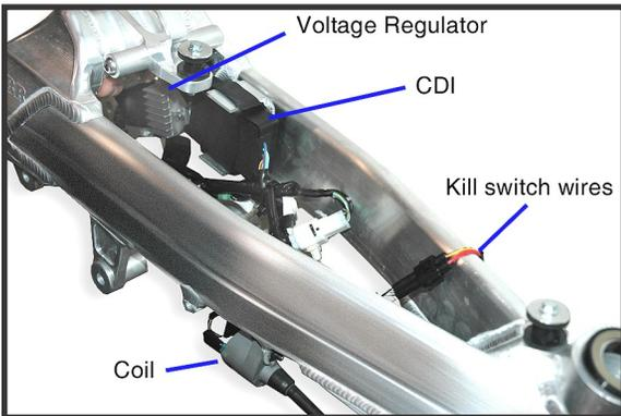
**4.** Install wire harness onto frame. Start with the voltage regulator. It bolts to a post on the left side under the shock tower with wires facing towards shock. Install CDI box on left side with wires facing forward. Install coil mount (with ground wire) with spark plug wire facing forward. Route the kill switch wire over the top of the left spar tube (just below gas tank mount).
