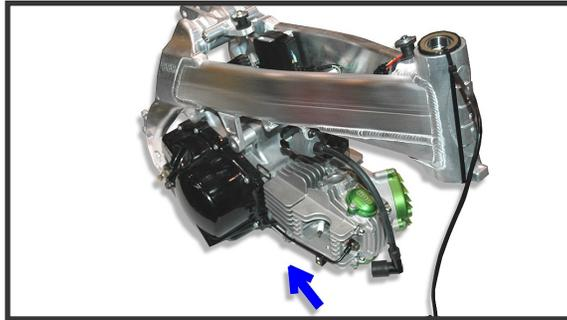
**5.** Install motor by sliding up into frame centering bottom motor mount plate between the bottom frame spars.
