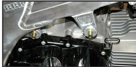
**6.** Install the top two motor mount bolts from the left side.
