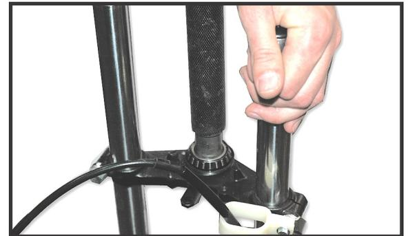
**10.** Install lower race for the tapered roller bearings on your steering stem. Be sure to remove the stock bearing race first.
