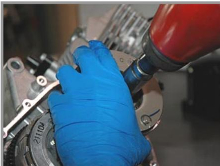
3. Use an impact wrench to remove the 19mm nut securing the primary clutch to the end of the crankshaft.
