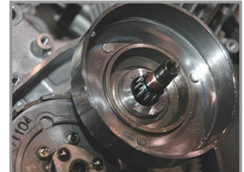
8. Slide the BBR Clutch Removal washer onto the end of the crankshaft (as shown above).
