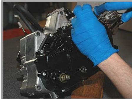
2. Remove clutch side cover (9 phillips head screws).
