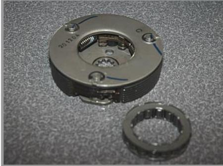
12. Shown here are the primary clutch shoe linings and the one-way clutch bearing that you will not reinstall.
