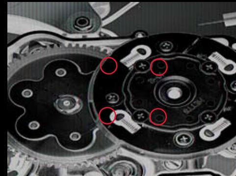
**15.** Straighten the tab of the clutch lock nut lock washer. Remove the clutch lock nut with the appropriate special clutch tool. It is available from Honda as part #07716-0020100.
