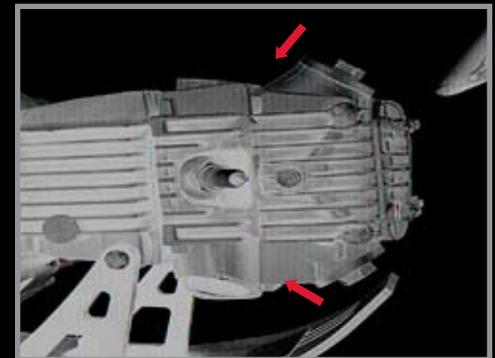
**29.** Install new oil pump onto the crankcase while aligning the pump shaft groove with the pump drive shaft. Install and tighten the (3) Phillips head screws that secure the oil pump.
