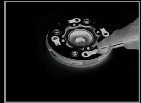
**34.** Reinstall the clutch assembly onto the crankshaft. Install the 14mm tabbed lock washer, then the conical lock washer (with the words "OUT SIDE" facing out), and then the lock nut. Use the special clutch tool to torque the nut to 31 ft. lbs.
