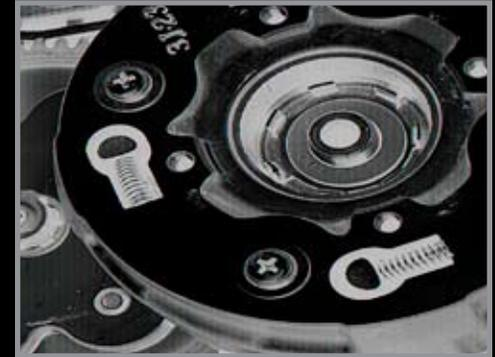
**35.** Install the clutch lifter cam plate, the "oil-through-spring" and "oil-through-tube". Next install the spring, ball retainer, and the clutch lifter arm. Finally, reinstall the clutch cover (right side engine case), kickstarter and brake pedal. Assembly is reverse of disassembly.
