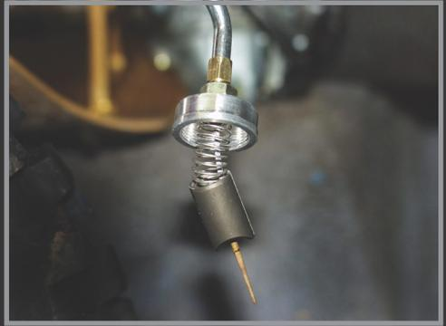
10. Install the slide into the carburetor. Make certain that the slide is facing the correct direction (as shown) when inserted into the carburetor. If it is inserted the other way, it will not seat all the way into the carburetor, and the motor will not idle down when started.
