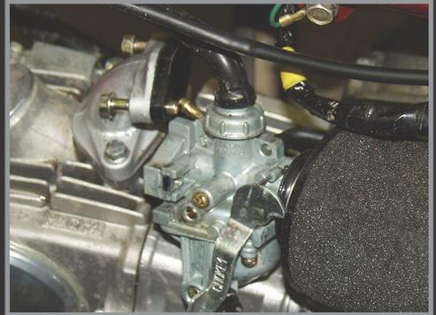
2. Remove the slide from the carburetor by unscrewing the carb top. Also remove the slide from the cable this time. This is done by compressing the spring and unhooking the cable from the bottom of the slide.
