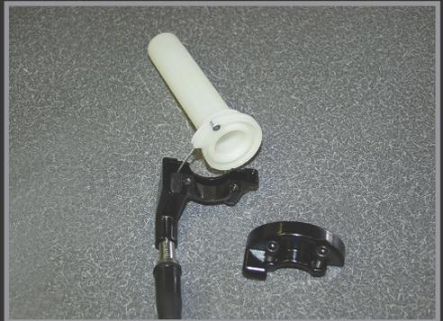
9. Install the slide and spring onto the new cable and carburetor top. If you cannot get the cable hooked into the slide with your fingers, try using needle nose pliers. Install the throttle tube onto the new handle bars.
