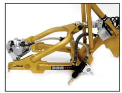
6. Slide caliper and mount into place on the swingarm. Zip ties can be used to secure the hoses out of the way.
