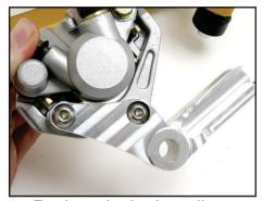
5. Replace the brake caliper mount with the one included in this kit. It will rotate the caliper back for more clearance. This is only necessary for a standard OEM style of swignarm.
