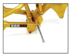
2. Remove the swingarm bolt to allow installation of the adapter plate.
