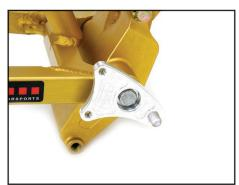
3. Install the master cylinder adapter plate as shown. It should fit over the new longer rear motor mount bolt.
