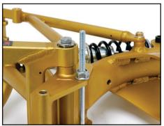
1. Replace the lower rear motor mount bolt with the long bolt supplied in this kit. This photo shows the bolt in place (with motor removed for easier view).
