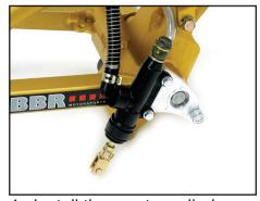
4. Install the master cylinder using the supplied 6mm bolts. The nylock nut should now be placed over the longer motor mount bolt. Tighten only until the nylock nut bottoms on the aluminum adapter. Do not over tighten or you will bend the adapter plate!
