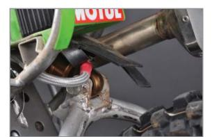
Installed correctly, the side panel will cover most of the reservoir.
