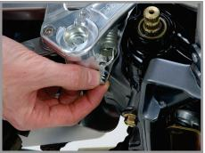
6. Adjust the brake pedal tip height as desired and lock the adjuster bolt in place.
