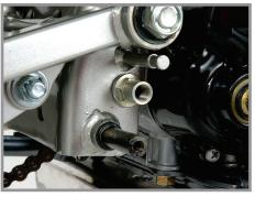
2. Replace the lower rear motormount bolt's nut with the special nut included in this kit (torque to 40 ft. lbs).
