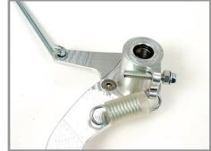
4. Hook brake pedal spring on the brake pedal. Install the stock o-rings in the BBR pedal.
