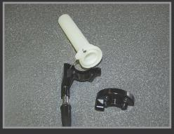
9. Install the slide and spring onto the new cable and carburetor top. If you cannot get the cable hooked into the slide with your fingers, try using needle nose pliers. Install the throttle tube onto the new handle bars.
