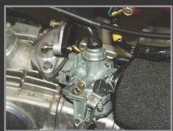
2. Remove the slide from the carburetor by unscrewing the carb top. Also remove the slide from the cable this time. This is done by compressing the spring and unhooking the cable from the bottom of the slide.
