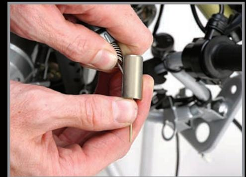
9. Remove the front brake cable by unthreading the adjuster at the bottom of the front brake mechanism. Use a 12mm wrench to remove the cable lock nuts from the fork.
