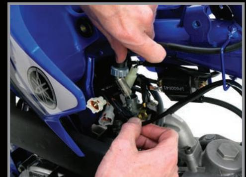
8. Pull back the spring and then unhook the carb cable from the carb slide. Retain the spring, slide, and needle for use with the BBR cable and carb top.
