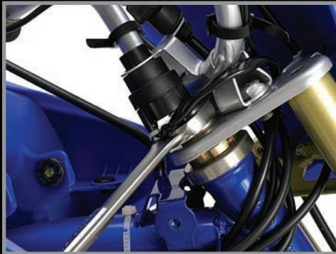
12. Cut the zip-tie holding the cables and wires to the frame, and you should now be able to remove the entire handlebar assembly.
