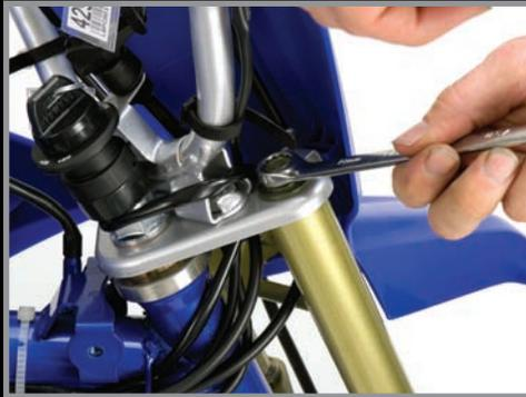
11. Use a 27mm wrench to remove the steering stem lock nut. If you remove the plastic lock nut that holds on the ignition key switch, it will give you enough room to remove the nut without removing the handlebars.
