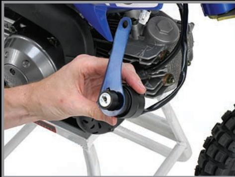
20. The key switch bracket mounts to the front coil screw. Remove the 8mm head screw and reinstall with the bracket.
