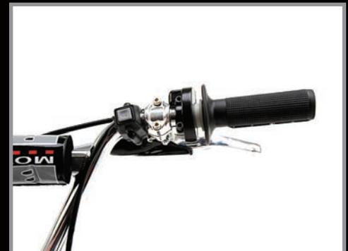
17. Install the brake lever on the right side of the handlebars. Install the start button also.
