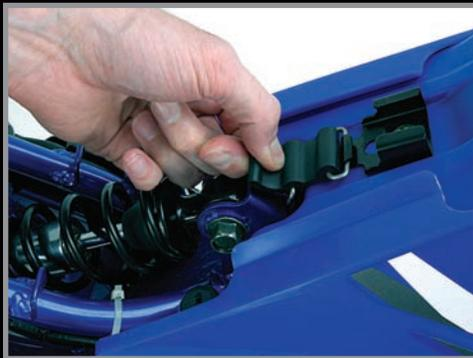
4. It is not necessary to remove the gas tank. You can access the carb by sliding the gas tank back as shown in the picture.
