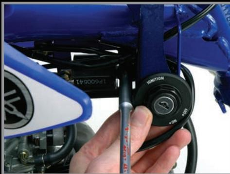
5. Disconnect the gray and white plugs just above the carb. The gray connector is for the kill switch. The white connector is for the starter button.
