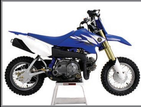
2. Remove the seat/rear fender/side panels by removing the (2) ten millimeter bolts under the rear fender.
