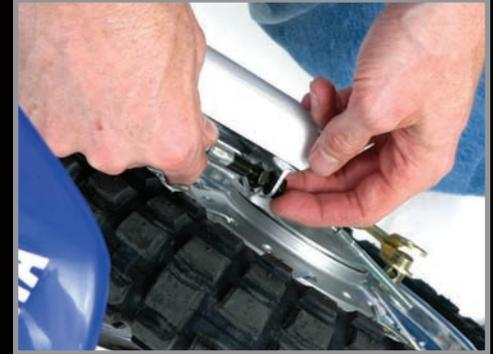
23. Reassemble the cable on the brake in the same manner as stock cable. Adjust brake as desired.
