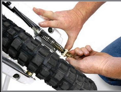
10. Remove the (2) 14mm head bolts at the top of the fork legs. If you do not support the front wheel, it can drop down once these bolts are removed.
