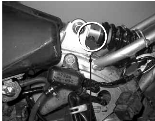
Picture #1: The rebound adjuster should face towards the left side of the bike. You might need to rotate the top eyelet to achieve proper positioning.
