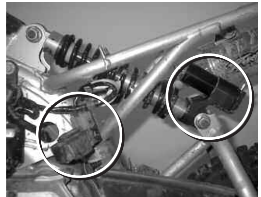
Picture #2: Reservoir end should face towards the rear of the bike. The CDI (rev box) should be moved to the location as shown.
