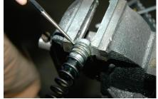
6. Screw the new springs onto the aluminum spring retainer by hand. Be certain that they are fully screwed on. Reassemble this fork leg and repeat procedure for the other fork leg.
