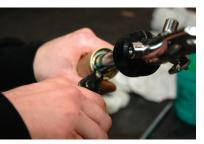
3. The lower fork leg should now pull apart( as shown at the left) We recommend wiping excess grease from the spring assembly to ease handling.
