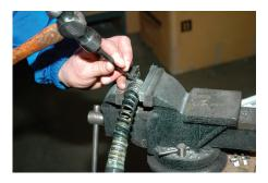
5. Clamp the aluminum spring retainer in a soft-jaw vice. Using an appropriate punch, unscrew the spring by striking the end of the spring wire. Once it has been loosened, it should unscrew by hand. Repeat procedure for the other end of the spring.
